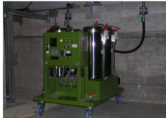
KLEENTEK ELC-R200SP-H on GE FR9FA gas turbine.
